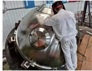
(c) 耐压壳焊接
