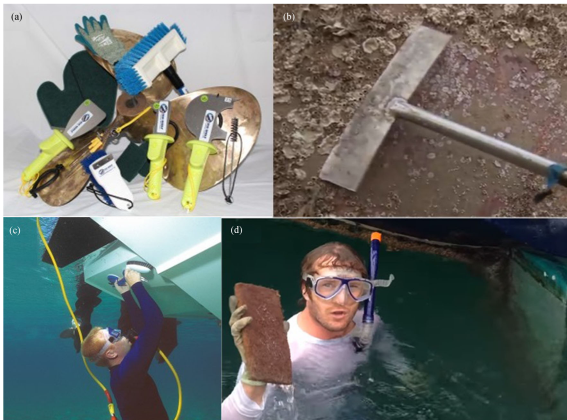
Figure 3 Manual hull cleaning tools and methods. a The cleaning tools provided by Top Shelf Marine Company (image: www.topshelfmarine.com/hull-and-bottom-cleaning ). b A shovel for removing barnacles (video screenshot: tv.cntv.cn/video/C10595/1a24d1bb3c7e453d8fa9183e8d62de44 ). c A diver using a handheld brush to clean the bottom hull (image: Citimarine Store , https://citimarinestore.com/citiguide/hookah-dive-systems-perfect-for-cleaning-hull-underwater/ ). d A snorkeler using a cleaning sponge to remove biofouling organisms (video screenshot: www.youtube.com/watch?v=0biZ4ysKHM0 )
