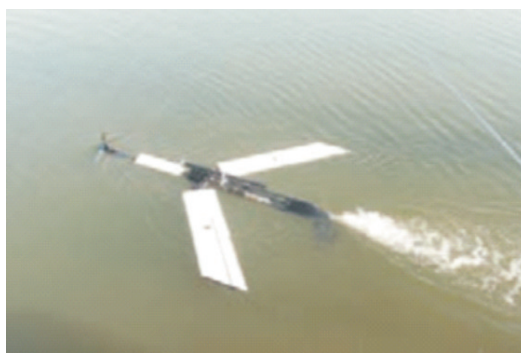
图18 北航仿鸬鸟潜空两栖跨介质无人飞行器 [49] Fig.18 Submersible UAV "Gannet" developed by Beihang University
