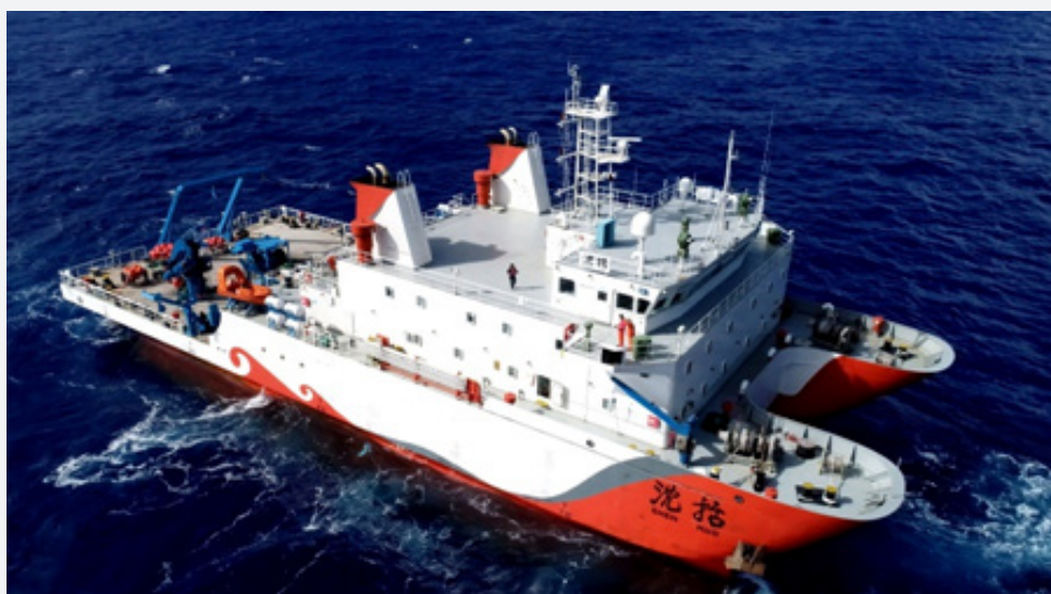
Figure 6: 2200-ton displacement SWATH type research vessel “Shen Kuo”.
