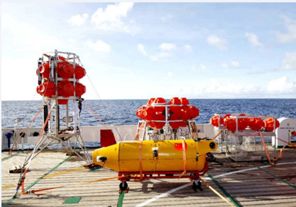
Figure 8: The first phase of the movable laboratory completed in Dec.2016 (three FOD landers and one FOD ARV prototype).
