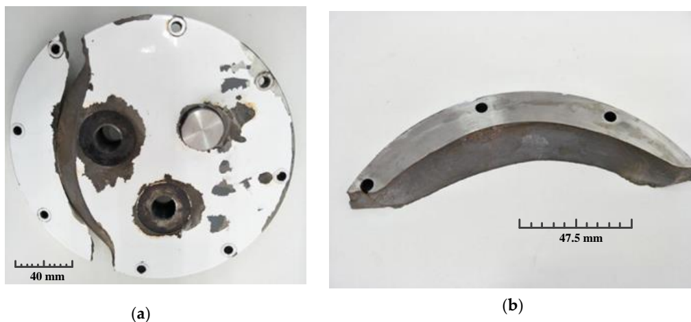
Figure 5. Photography of the cracked flat cover: (a) upper surface of the cover; (b) fracture surface in the outer edge of the cover.
